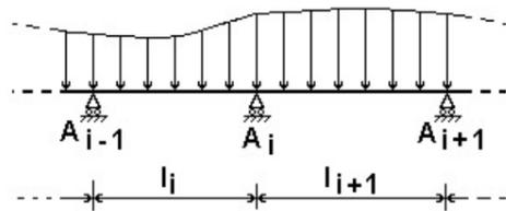
$$M_{i-1} \frac{l_i}{6EI} + M_i \frac{l_i}{3EI} + \frac{l_{i+1}}{3EI} M_i + M_{i+1} \frac{l_{i+1}}{6EI} = \omega_{i+1}' - \omega_i''$$
