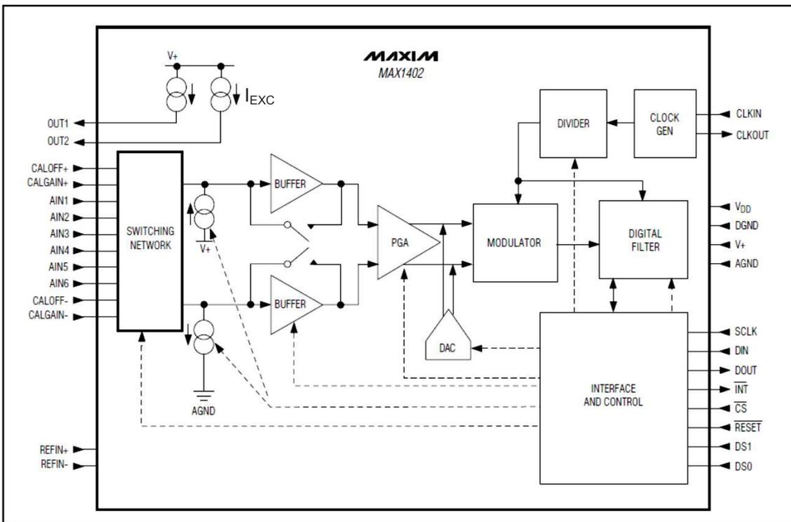
Figure 2. Functional Diagram
