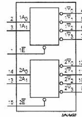
Fig.4 Functional diagram.
