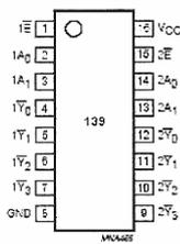
Fig.1 Pin configuration.
