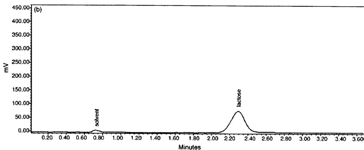
Effect of impactor setting on sensitivity. Chromatograms of lactose ( $1 \text{ mg.mL}^{-1}$ ) using (a) impactor "off" and (b) impactor "on" (optimized conditions  $90^\circ\text{C}$  and  $3 \text{ L.min}^{-1}$ ).
